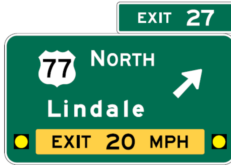
Exit Direction sign with E13-2 sign panel and flashing yellow beacons
