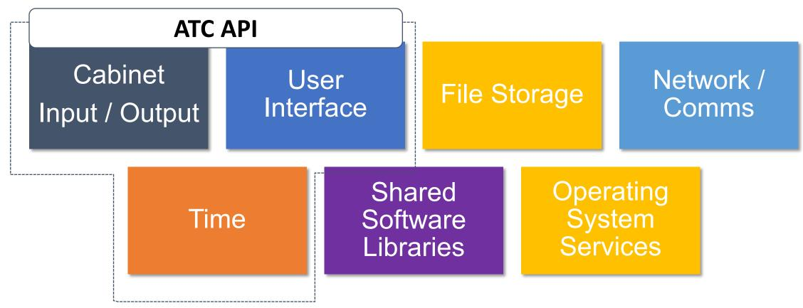
ATC 5401 - focused on these three subsystems Application Programming Interface
